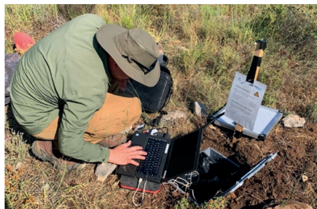
Installation of a seismic sensor: The team is measuring the slightest vibrations throughout the area of the Methana Volcano. (Photo: Jan-Phillip Föst)
