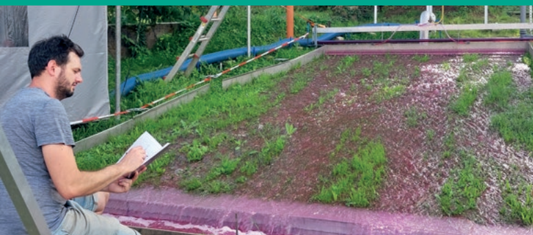
Field experiment with tracer dye on a sloping meadow – with the mobile test bed, the team is simulating real-life extreme rainfall scenarios. (Photo: KIT-IWU / Peter Oberle)
