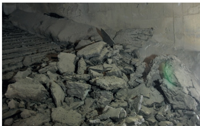
When it's too late: Slag and loose deposits from a biomass furnace – disposal required. (Photo: Kolb / KIT)
