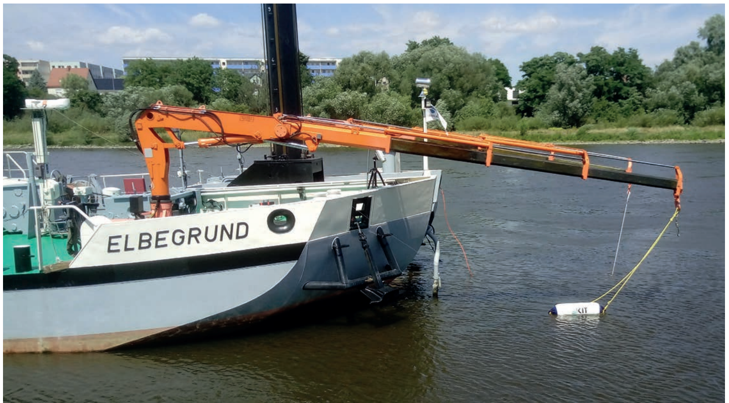
The Elbe river is a real-world lab for studying the precision of hyperspectral measurement methods: Measurement boat with hyperspectral sensor and parallel sampling. (Photo: Keller, S. et al., Hyperspectral Data and Machine Learning for Estimating CDOM, Chlorophyll a, Diatoms, Green Algae and Turbidity , Int. J. Environ. Res. Public Health 2018, 15(9))
