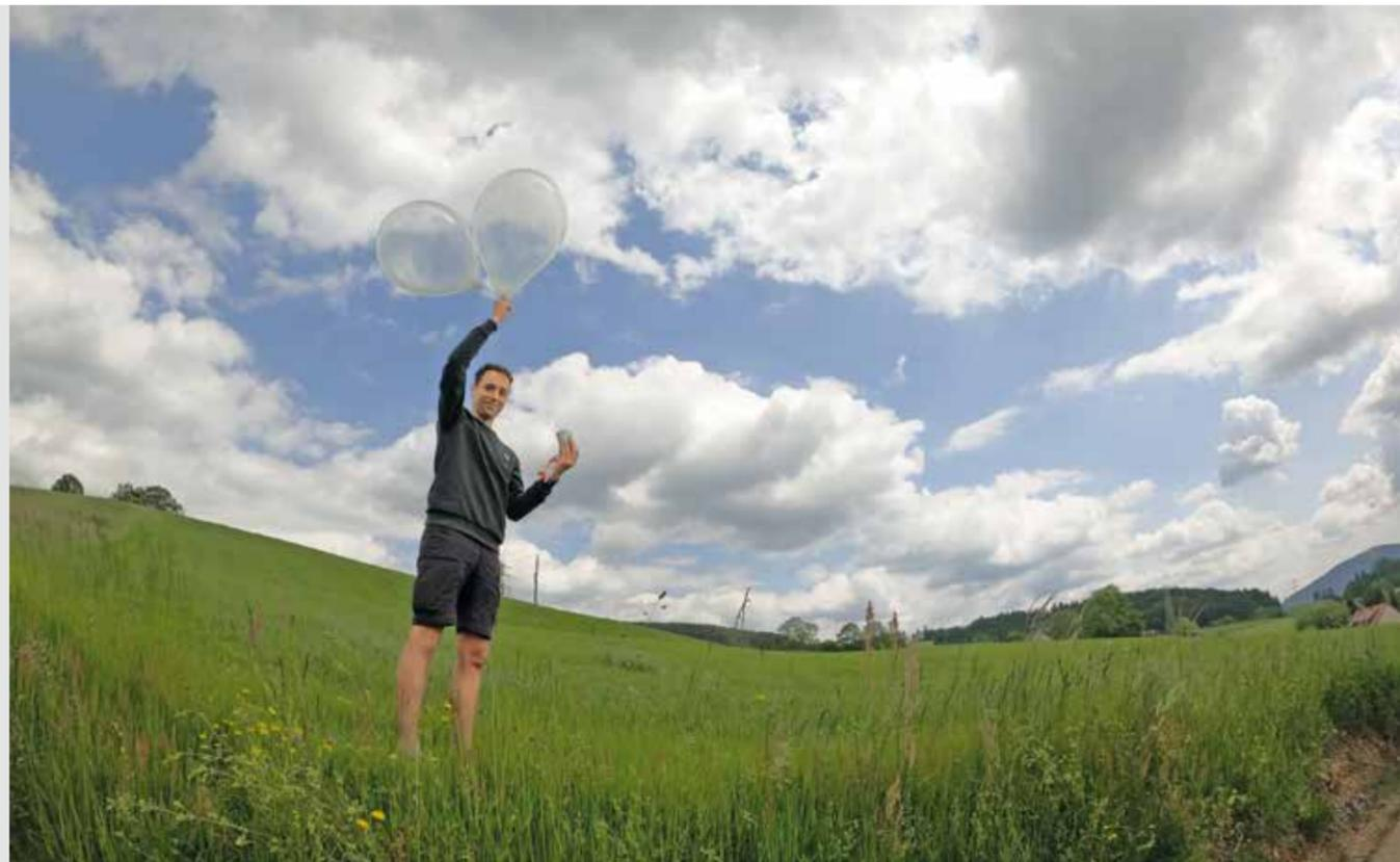
Exact weather forecasts and good scientific instinct allow helium-filled balloons to carry the measuring sondes directly into the storm cell. (Photo: Kunz)
