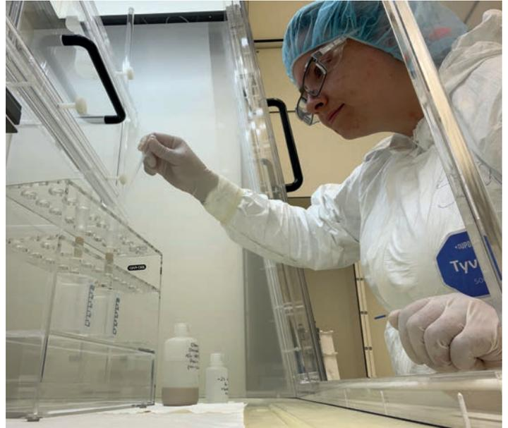
Dr. Sara Kimmig prepares ion exchangers used for the chemical purification of potassium for isotope analysis. (Photo: S. Kimmig, KIT)
