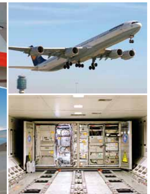
IAGOS-CARIBIC A340-600 of Lufthansa with air inlet system (left) and laboratory of 1.6 t in weight (bottom right), which is installed into the cargo compartment for automatic measurements during four flights per month. (Photos: Kröner/Lufthansa AG (left), Lufthansa AG (top right), MPI for Chemistry (bottom right))
