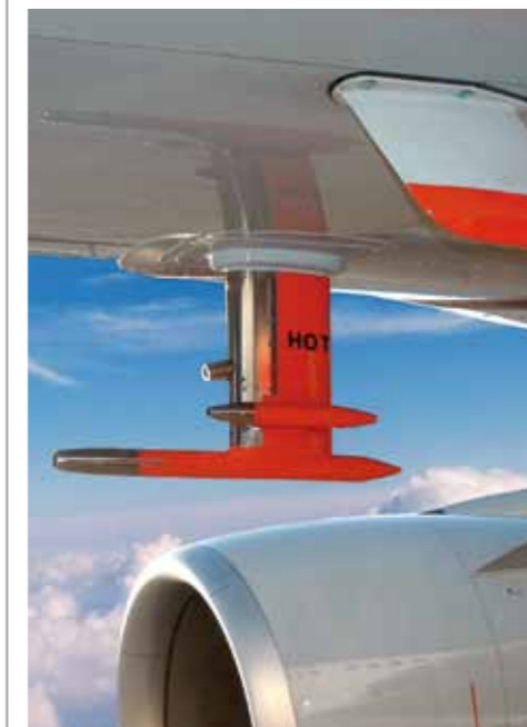
IAGOS-CARIBIC A340-600 of Lufthansa with air inlet system (left) and laboratory of 1.6 t in weight (bottom right), which is installed into the cargo compartment for automatic measurements during four flights per month. (Photos: Kröner/Lufthansa AG (left), Lufthansa AG (top right), MPI for Chemistry (bottom right))
