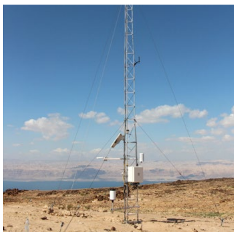
Water loss on the Dead Sea: With the help of such measurement stations, KIT researchers determine the extent of evaporation. (Photo: KIT/Corsmeier)
