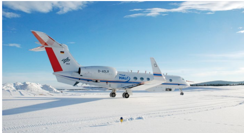
HALO waiting for the start in Kiruna. On top of the fuselage, a number of air inlets for in-situ measurement instruments can be seen. The GLORIA infrared spectrometer is visible underneath. (Photo: Björn-Martin Sinnhuber)
