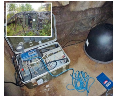
Many measurement stations of this type measure seismic waves. (Photo: Michael Grund)
