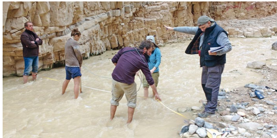
Discharge measurement under flash flood conditions. (Photo: Maren Haid / KIT)
