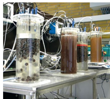
The four laboratory reactors used for studying deammonification. (Photo: Susanne Lackner, KIT)
