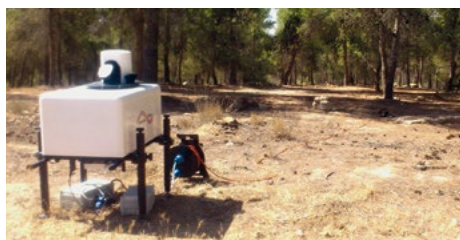
The Doppler lidar (left) is used to measure how air flows ascend above the forest and how they affect the boundary layer of the atmosphere. (Photo: Matthias Mauder)
