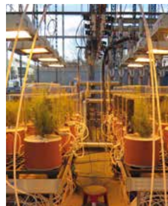
In automatic measurement chambers, Aleppo pines were exposed to increasing temperatures. (Photo: Plant Ecophysiology Lab, KIT)
