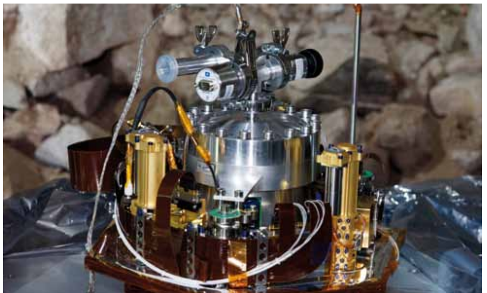
The Mars seismometer tested in the BFO tunnel: the vacuum chamber with the sensors is positioned between three motorized foot screws (only two are visible). With these screws, the seismometer is leveled. (Photo: Philippe Labrot, IGP, Paris)
