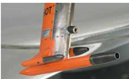
Via an inlet system, air and aerosol samples are taken during the flight. (Photo: Stefan Weber)
